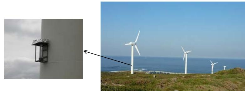
**Fig. 1** - Atmospheric testing corrosion station.
