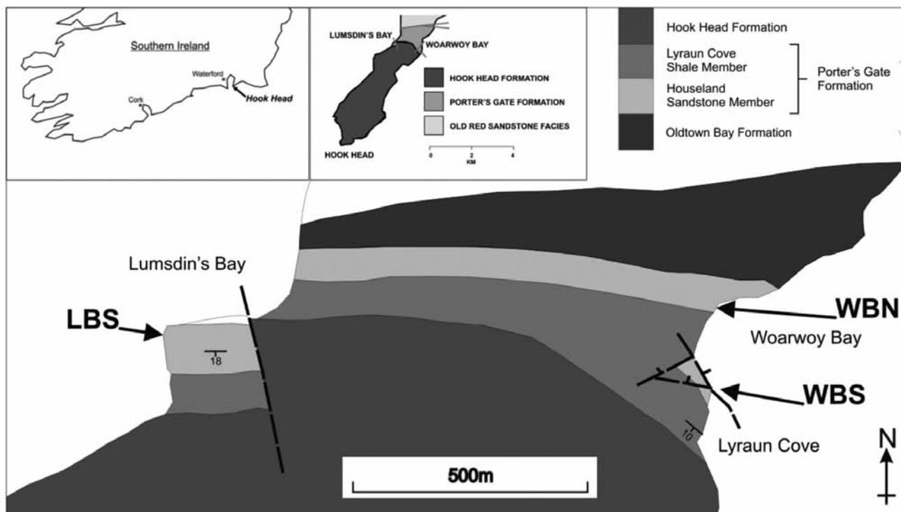
Fig. 1 – Map of the Porter's Gate Formation showing the locations of the three sections logged and sampled at Woorwoy Bay North (WBN), Woorwoy Bay South (WBS) and Lumdsin's Bay South (LBS), adapted from SLEEMAN, 1977 and GARDINER & HORNE, 1981.
